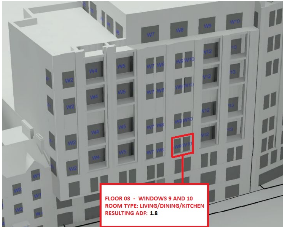
Figure 22 (above): Window map of the Southwark Fire Station redevelopment, highlighting the one room that would experience a loss of ADF to less than the level advised by the BRE guidance.
