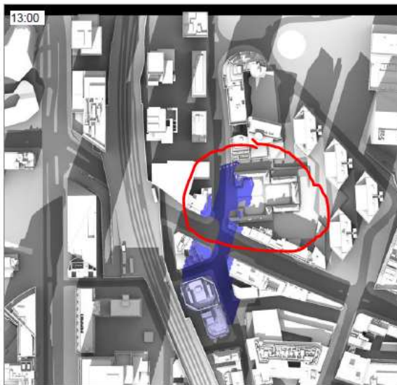
Image showing existing premises (green) and the proposed development (blue) and the amount of overshadowing on March 21 st at 13.00
